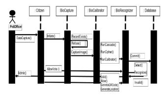
Figure 18. UML interaction sequence for Election Authentication.
