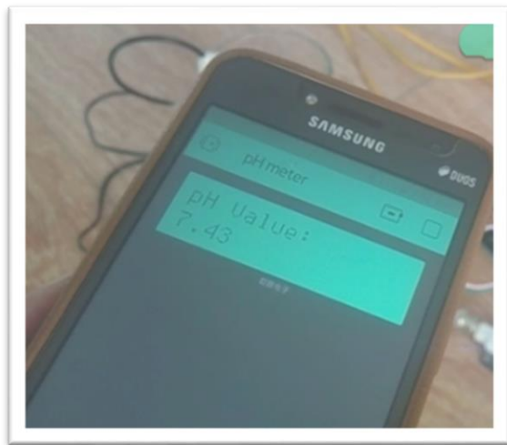
Fig 17: The pH meter monitored through the mobile phone.
