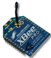
Figure 2: ZigBee Module from Digi International Inc. (19)
