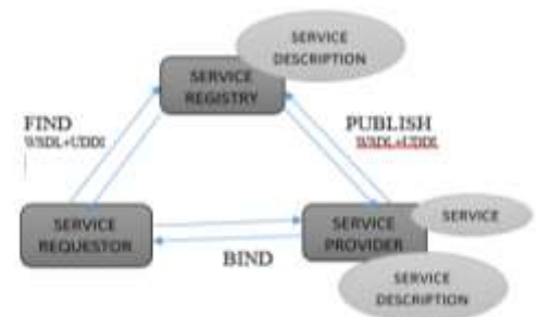
FIGURE 1: web service architecture
