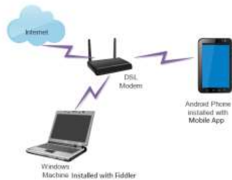
Figure 2: Network setup using fiddler as a proxy on windows machine
